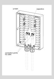
Mark adjusted Capacitor Boxes with the value that they are adjusted to on outside in the designated space on the type plate.
