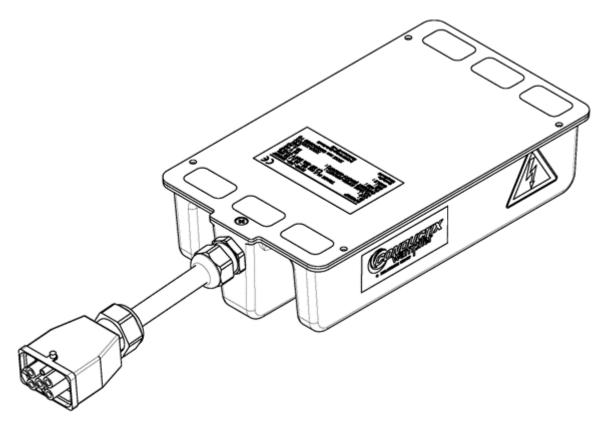
Drawing shows pickup with straight cable outlet.
