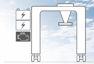
In Conductix-Wampfler Hybrid RTG systems the battery pack is the main power supply and connected through a very efficient DC/DC converter to the DC bus of RTG drive.
